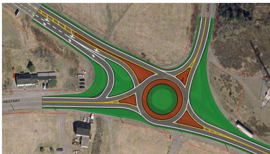
Exhibit 3.5: Manawagonish Road/Gault Road Single Lane Roundabout
