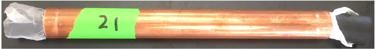
Figure 1: A section of new copper pipe sealed at either end with a rubber stopper.
