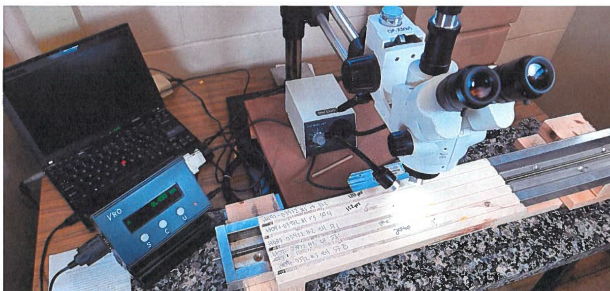
Figure 2. Velmex stage measuring system with a sample. Photo cr: Ben Phillips
