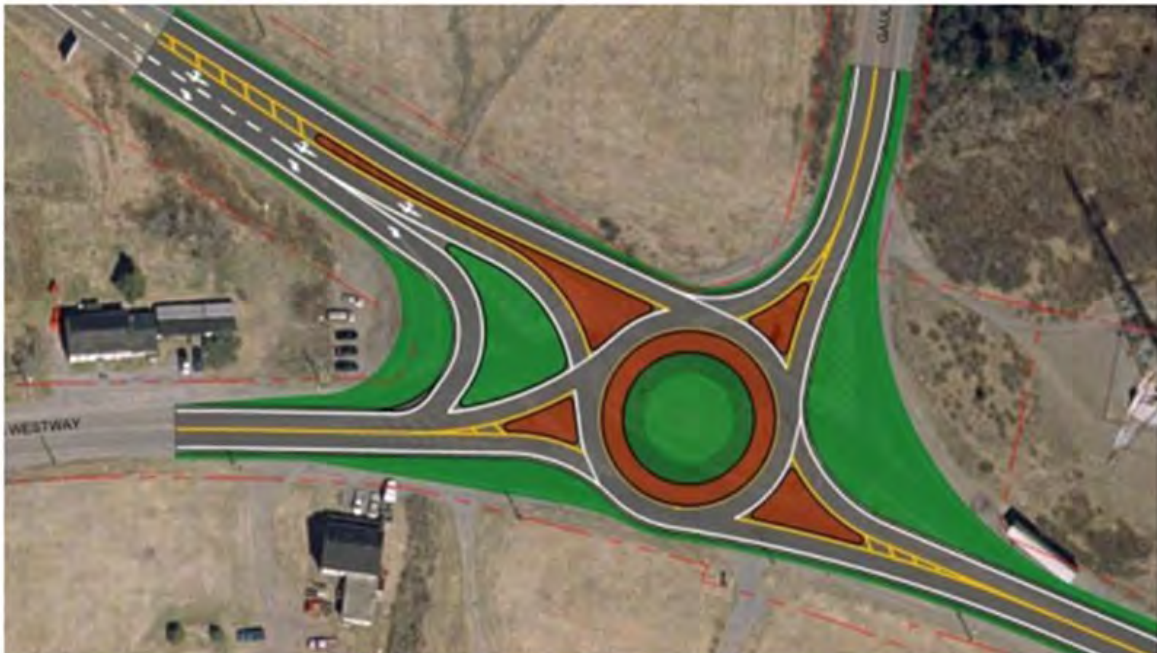
Exhibit 3.5: Manawagonish Road/Gault Road Single Lane Roundabout
