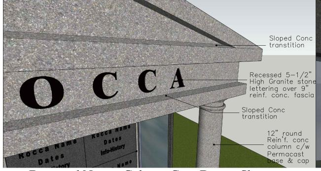
Recessed Name- Column Cap- Recess Slopes 3D View A1-13
